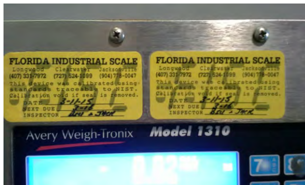
The test bench scale was certified to be calibrated according to National Institute of Standards and Technology (NIST).
