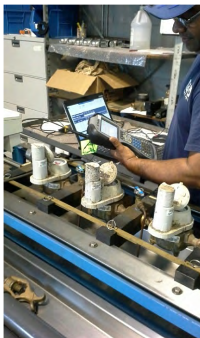
Testing the transmitter reads with a handheld reader to verify the read on the meter register.
