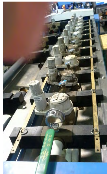
The test bench with meters loaded for testing.
